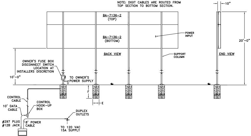
COLUMNS AND FOOTINGS SHOWN HERE, PROVIDED BY OTHERS, ARE SIZED TO COMPLY WITH IBC 2006 90 MPH EXPOSURE B REQUIREMENTS. THE MANUFACTURED PRODUCT EXCEEDS THE REQUIREMENTS OF IBC 2006 90 MPH EXPOSURE B AS MOUNTED IN THIS DRAWING. SOIL— AVERAGE WITH ALLOWABLE STRESSES OF 2500 psf. DESIGN SHOULD BE ALTERED FOR DIFFERENT SOIL CONDITIONS, CLEARANCE, OR LOCAL CODES. FAIR—PLAY ASSUMES NO RESPONSIBILITIES FOR INSTALLATIONS DONE BY OTHERS.
