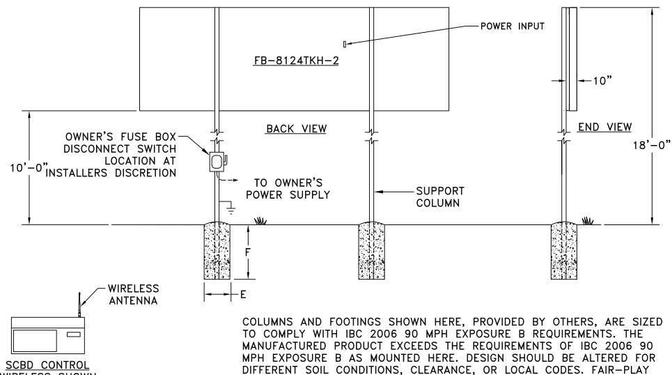
CONTROL CABLES- SUGGEST 1/2" CONDUIT BE USED FOR BURIED CABLE IN AREAS WHERE IT MAY BE SUBJECT TO MECHANICAL DAMAGE. POWER WIRES SHOULD BE ROUTED IN SEPARATE CONDUIT FROM CONTROL CABLE.
