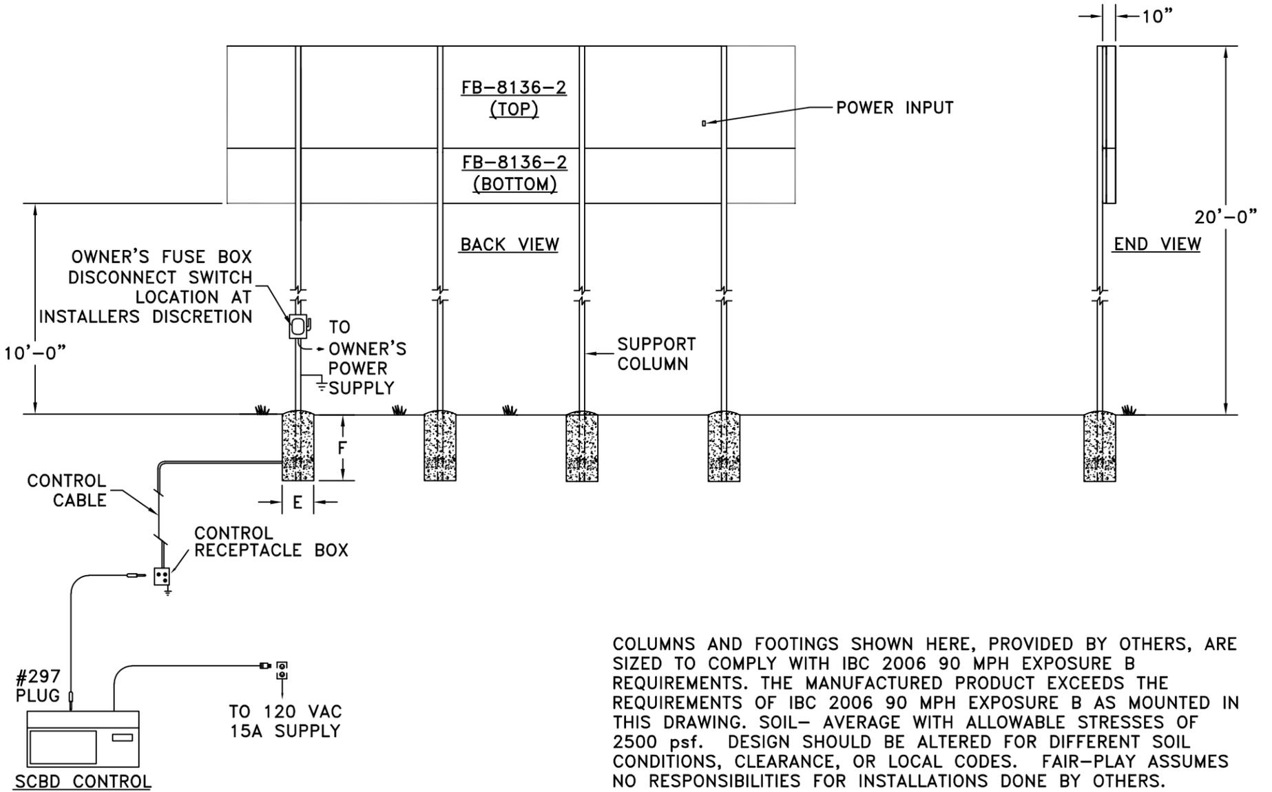
COLUMNS AND FOOTINGS SHOWN HERE, PROVIDED BY OTHERS, ARE SIZED TO COMPLY WITH IBC 2006 90 MPH EXPOSURE B REQUIREMENTS. THE MANUFACTURED PRODUCT EXCEEDS THE REQUIREMENTS OF IBC 2006 90 MPH EXPOSURE B AS MOUNTED IN THIS DRAWING. SOIL- AVERAGE WITH ALLOWABLE STRESSES OF 2500 psf. DESIGN SHOULD BE ALTERED FOR DIFFERENT SOIL CONDITIONS, CLEARANCE, OR LOCAL CODES. FAIR-PLAY ASSUMES NO RESPONSIBILITIES FOR INSTALLATIONS DONE BY OTHERS.
