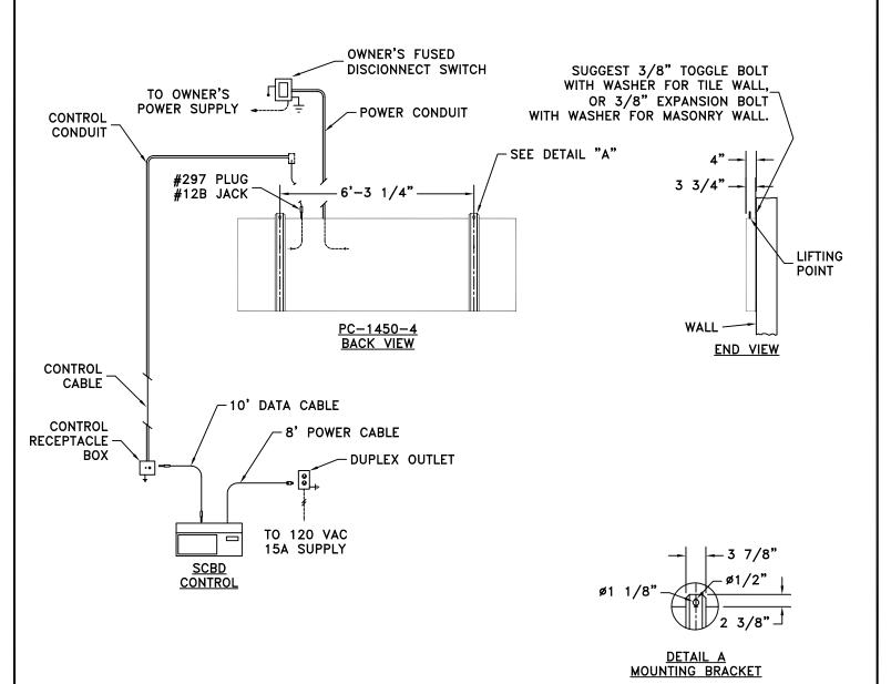
NOTES: POWER WIRES SHOULD BE ROUTED IN SEPARATE CONDUIT FROM CONTROL CABLE. SUGGEST 1/2" CONDUIT FOR CONTROL.
