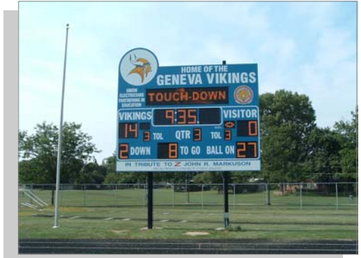
Geneva High School | Geneva, Illinois FB-8120TKH-2 football scoreboard 16x80, 1.75" (45mm) amber CaptiVue display
