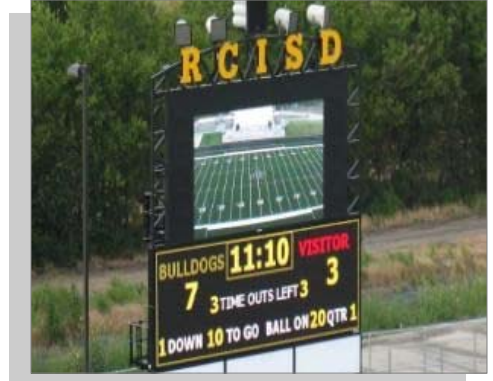
Royce City ISD | Royce City, Texas Custom Football matrix scoreboard 136 x 416, 0.9" (23mm) RGB CaptiVue display
